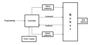
Figure 2: Block Diagram of General Purpose Robot
